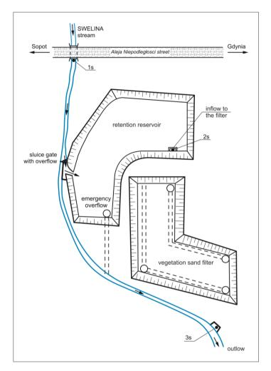
**Fig. 3.** The CW system on Swelina Stream, according to [11] **Rys. 3.** Object hydrofitowy na Potoku Swelina [11]
