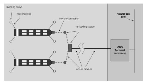
**Fig. 4.** Exemplary scheme of unloading CNG tanker at the open sea – own source
