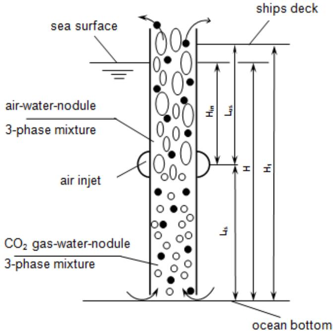
**Fig. 5.** Model of hydraulic with air-injector transportation of poly-metallic concretions
