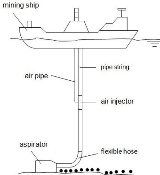
**Fig. 3.** Idea of HPWJ-mining and hydraulic transportation of concretions using air-injector
