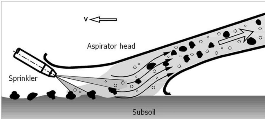
**Fig. 4.** New working system (aspirator head) of concretions sucking
