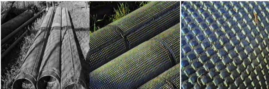
Fig. 4. Slotted stainless steel filter extracted from well bottom after 75 years of its exploitation
