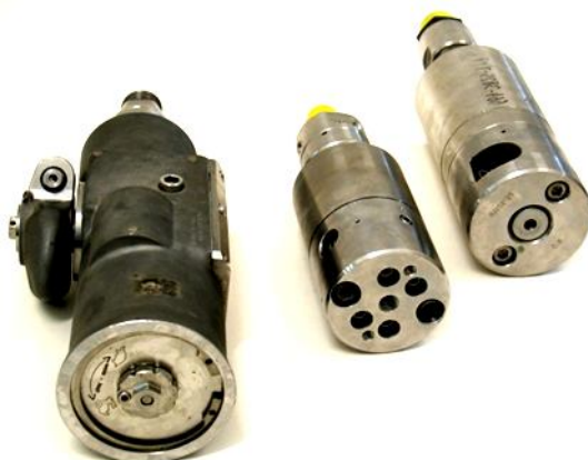
Fig. 5. Different rotary working heads types used for high-pressure water jet wells cleaning
