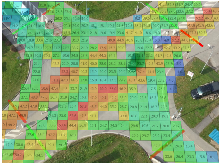
Fig. 7. Average speed visualization – grid map using the DataFromSky application. Source: authors
