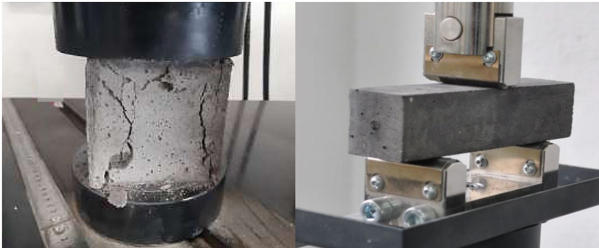
Fig. 1. Samples and setup for compressive and flexural strength
