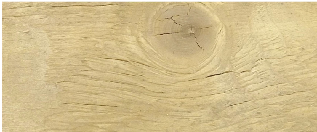
Fig. 3. Cracks in the outer layers of aged LVL specimens
