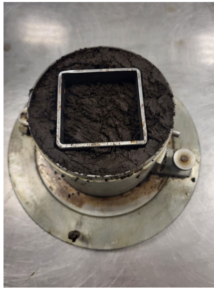
Fig. 3. Scheme of taking a composite material by cutter from the lower cylinder of the Proctor apparatus
