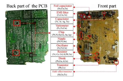
Fig. 2. Identification of the elements present in the isolated PCB
