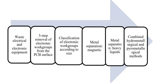
**Fig. 5.** A sample scheme of waste material flow which enterprises should use in their plants
