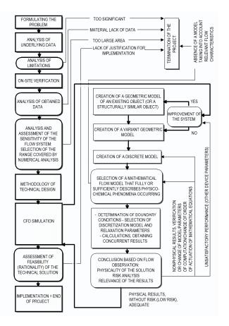
Fig. 3. Scheme for the design and modernisation of machines and flow-through systems using CFD software
