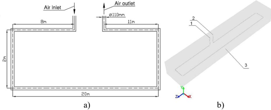
**Fig. 6.** Geometric dimensions of the heat exchanger (b) and scheme of the calculation area (a): 1 – air inlet to the EAHE; 2 – air outlet from the heat exchanger; 3 – soil mass
