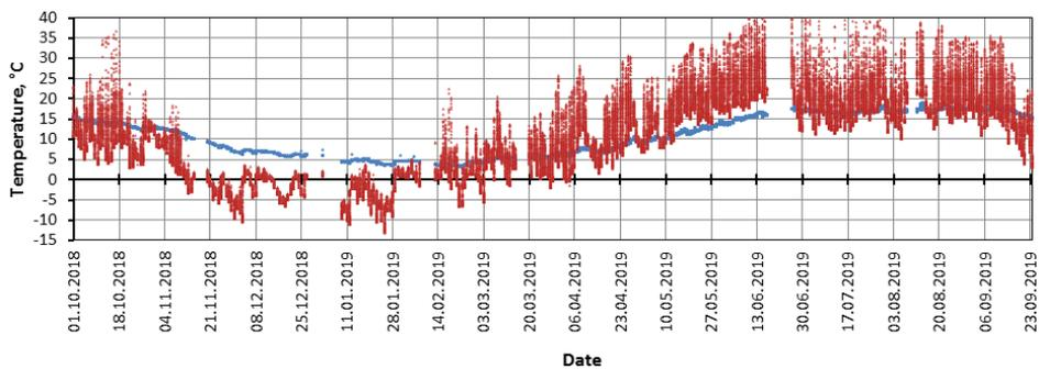
**Fig. 2.** Experimental data for ventilation air temperature (red drops – air inlet in EAHE; blue drops – air outlet from EAHE)
