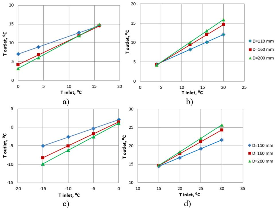
**Fig. 9.** Dependence of the air temperature at the outlet of the EAHE at various pipe diameters for: a) October; b) April; c) January; d) July
