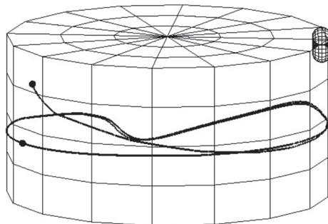
**Fig. 4.** Part of the quasi-stationary particle free settling path
