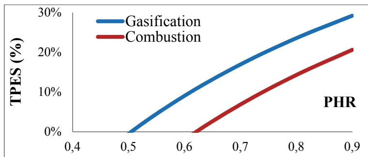
**Fig. 4.** Trigeneration primary energy saving depending on Power to Heat Ratio
