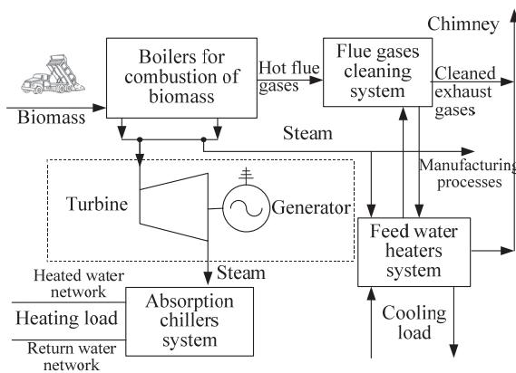
**Fig. 2.** Exemplary diagram showing the biomass combustion in a trigeneration system
