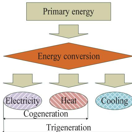
**Fig. 1.** Combined production of electricity, heat and cooling
