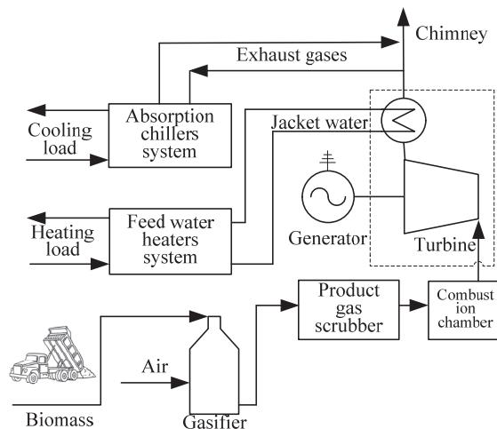
**Fig. 3.** Exemplary diagram showing the gasification of biomass in a trigeneration system
