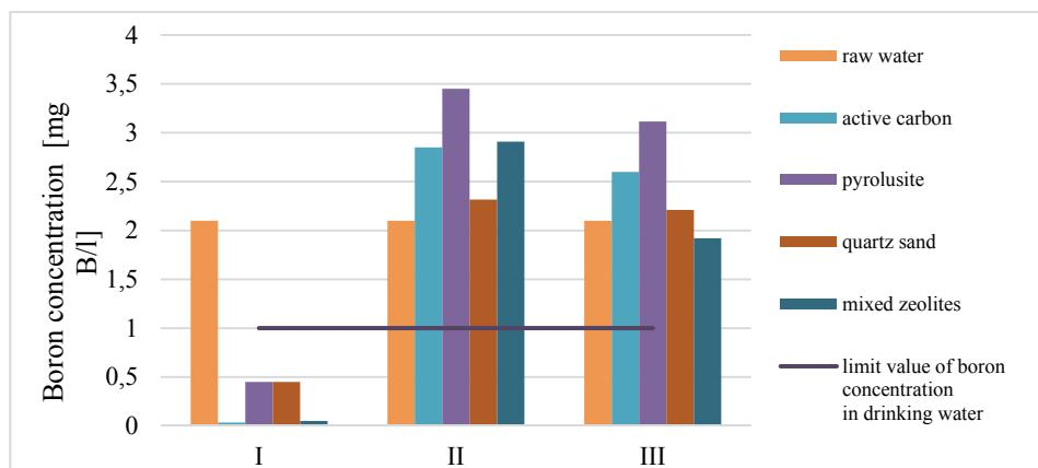
**Fig. 1.** Boron concentration in raw and filtrated water
