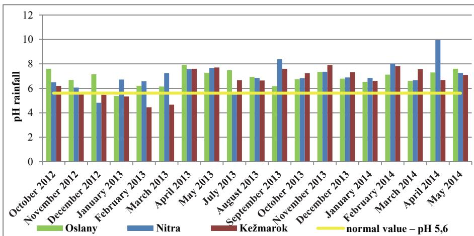
**Fig. 3.** pH parameters measured in 3 locations, yellow line represents pH 5.6
