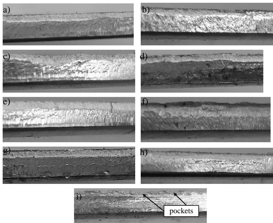
**Fig. 4.** Characteristic features of the sheared edges under study: a)  $v = 7$  m/min,  $c = 0.05$  mm, b)  $v = 27$  m/min,  $c = 0.05$  mm, c)  $v = 7$  m/min,  $c = 0.13$  mm, d)  $v = 27$  m/min,  $c = 0.13$  mm, e)  $v = 3$  m/min,  $c = 0.09$  mm, f)  $v = 32$  m/min,  $c = 0.09$  mm, g)  $v = 17$  m/min,  $c = 0.03$  mm, h)  $v = 17$  m/min,  $c = 0.15$  mm, i)  $v = 17$  m/min,  $c = 0.09$  mm
