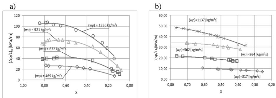
**Fig. 6.** The results of the experimental characteristics  $(\Delta p/L)_x = f(x)$  during the refrigerant R407C condensation in minichannels with internal diameter:
