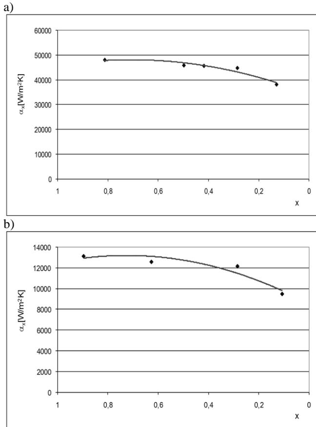
**Fig. 5.** Experimental results as dependence of  $\alpha_x = f(x)$  during condensation of R407C refrigerant in pipe minichannels with internal diameter: a)  $d = 0.31$  mm, b)  $d = 0.98$  mm
