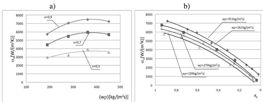
**Fig. 9.** Experimental results dependence of the average heat transfer coefficient  $\alpha_A$  on: a) mass flux density  $(w\rho)$  for  $x_A = \text{const}$ , b) the average vapour quality  $x_A$ , for  $(w\rho) = \text{const}$ , MULTI-8, R134a
