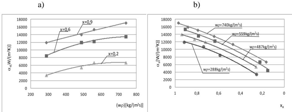
**Fig. 8.** Experimental results according to the average heat transfer coefficient  $\alpha_A$  from: a) mass flux density  $(w\rho)$  for  $x_A = \text{const}$ , b) the average vapour quality  $x_A$ , for  $(w\rho) = \text{const}$ ; MULTI-4, the refrigerant R407C
