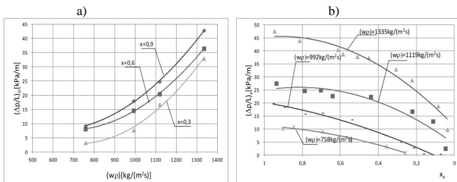
**Fig. 10.** Experimental results dependence of the flow resistance  $(\Delta p/L)_A$  of: a) mass flux density  $(w\rho)$  for  $x_A = \text{const}$ , b) the average vapour quality  $x_A$ , for  $(w\rho) = \text{const}$ .; MULTI-4, R404A
