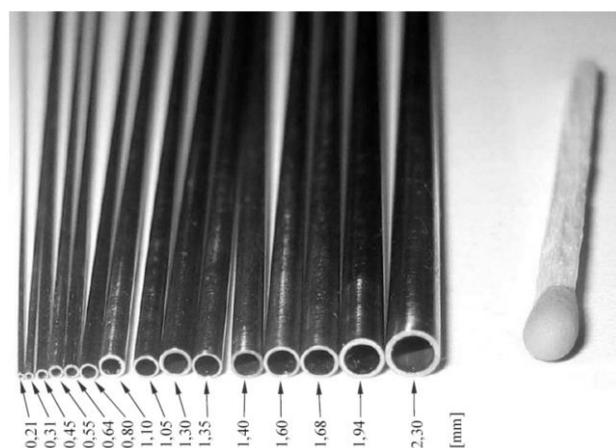
**Fig. 1.** View of the tubular mini-channels used for the purpose of the experimental research
