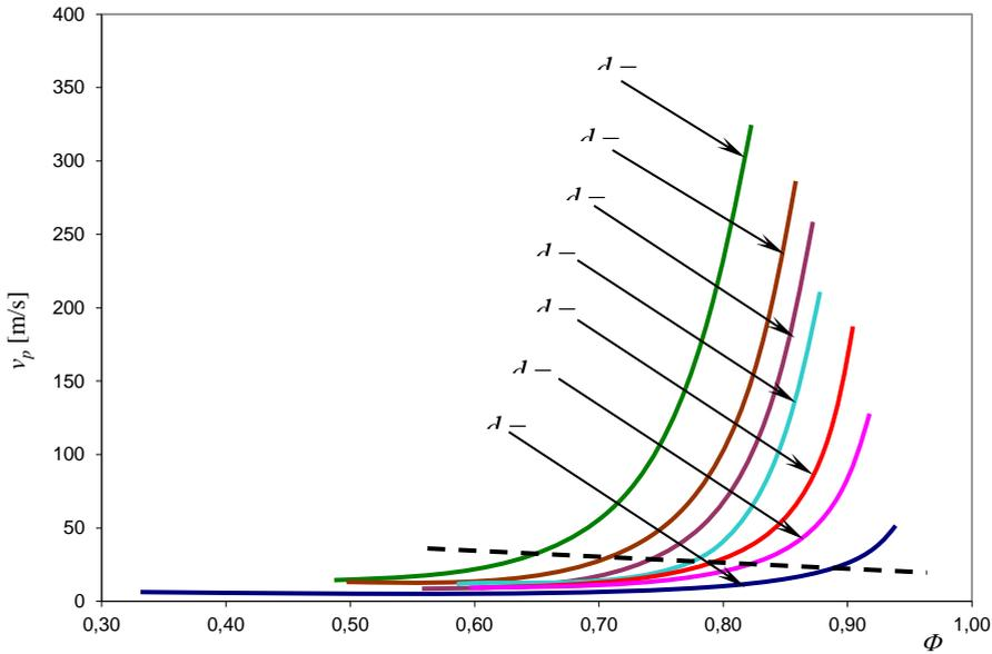
**Fig. 12.** Summary of experimental results characteristics  $v_p = f(\Phi)$  during condensation of refrigerant R134a in pipe minichannels with internal diameter  $d = 0.64, 0.90, 1.40, 1.44, 1.92$  and  $3.30$  mm in a periodic instability
