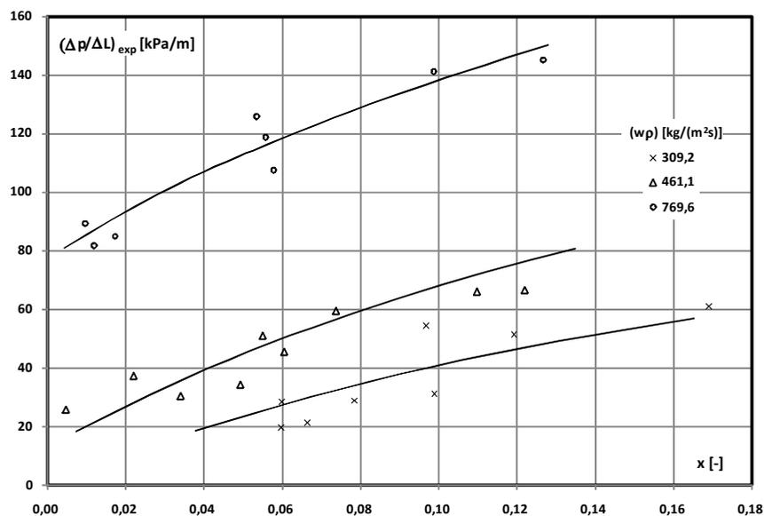
**Fig. 4.** Dependence of two-phase flow resistance on equilibrium vapour quality  $x$ ; R134a,  $d = 0.45$  mm,  $(w\rho) = \text{const}$
