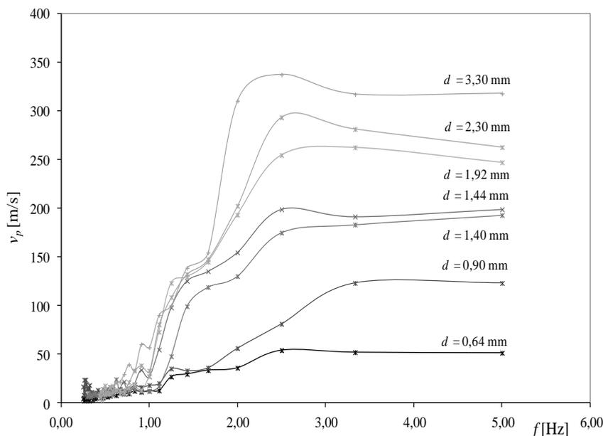
**Fig. 11.** Experimental dependant on the speed  $v_p$  of movement pressure instability of the periodic distribution generation during refrigerant R134a condensation in pipe minichannels of internal diameter  $d = 0.64$ – $3.30$  mm
