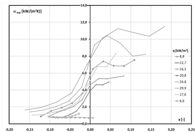
**Fig. 3.** Experimental dependence of local heat transfer coefficient  $\alpha_{exp}$  on equilibrium vapour quality  $x$ ; R134a,  $(w\rho) = 436.4 \text{ kg}/(\text{m}^2\text{s})$ ,  $d = 0.80 \text{ mm}$
