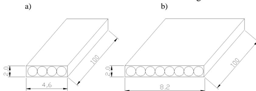
**Fig 7.** Dimensional diagram of tested minichannels bundles: a) MULTI-4, b) MULTI-8
