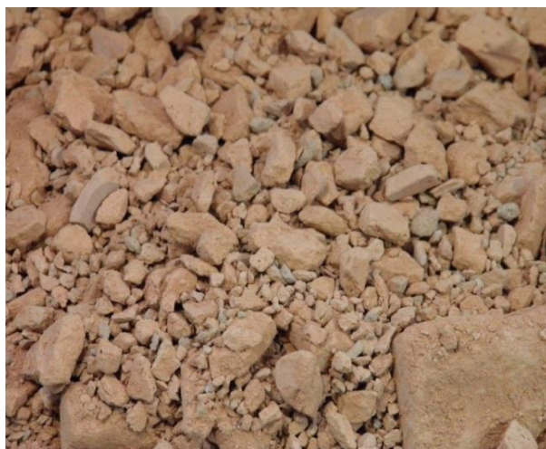
Fig. 1. Ground ceramic waste used as coarse aggregate
